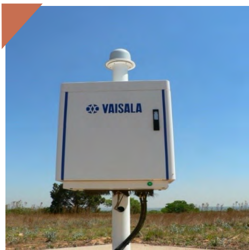
Lightning detectors form part of the SAWS Lightning Detection Network (LDN)
