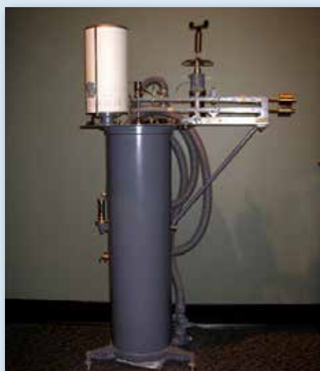
Figure 2. Dines pressure tube anemograph ( www.campbellsci.ca )
