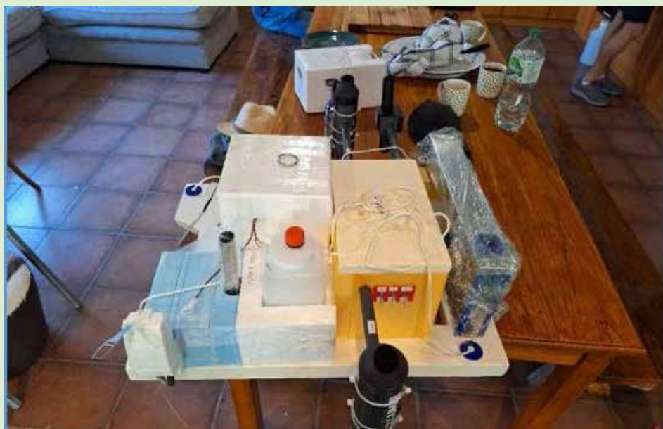
Figure 3: Instrument payload with NIXE (balloon) - a cirrus cloud ice particle imager on the far right of the image, UCASS (aerosol counter) in the middle of the image, CFH – Cryogenic Frost point Hygrometer (in light blue cover), ozone sonde with Vaisala radiosonde (top left box), LOAC – aerosol counter (in the middle of the table).
