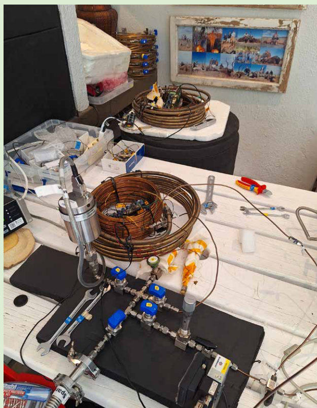
Figure 5: Temporary laboratory constructed inside Branddoorns Hunting Lodge, Beaufort West. Right depicts an AIRCORE atmospheric sample (coiled tube) pushed into a Picarro instrument shown on left side picture to quantify greenhouse gases such as carbon dioxide and methane.
